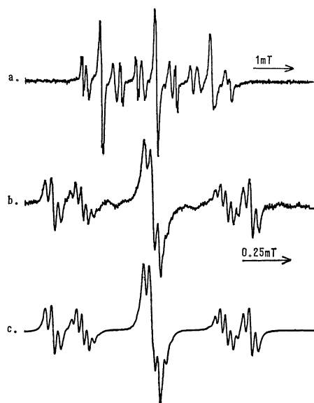
Fig. 3. (a) The ESR spectrum recorded when a NDCHA: ethanol solution containing di- t -butyl peroxide was photolysed at –10 °C. (b) The centre portion of the spectrum expanded. (c) The simulated ESR spectrum of (b) using the coupling constants in Table 3.
